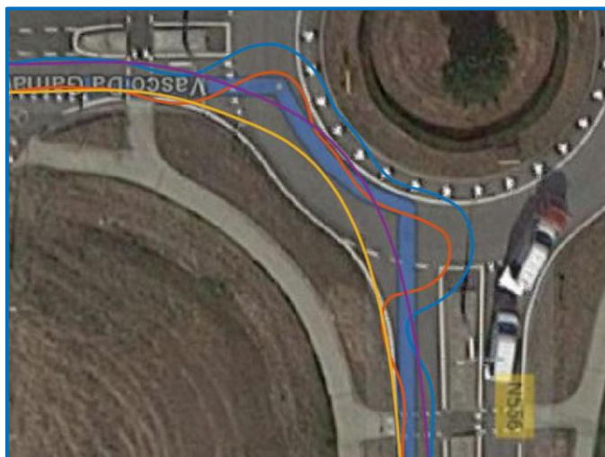
Figure 57: Critical Section #3 – Tyre outer walls envelope
